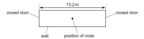
What is the lowest frequency of sound that could create a stationary wave in the corridor with a node halfway along it?
