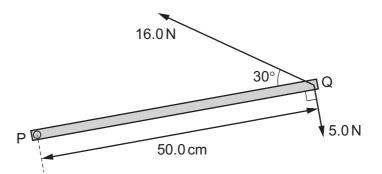
Two forces of 16.0 N and 5.0 N are in the horizontal plane and act on end Q, as shown.
