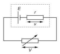
The resistance of the variable resistor is gradually increased from r to 3r.
